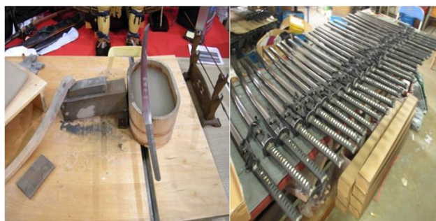
Figure 10. Traditional vs modern differential hardening for swords Source: Butouken Martial Art Swords & Samoerai Zwaarden Informatie
